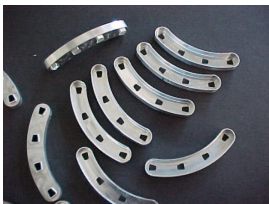
Open aluminum cooling containers after the difficult machining.
