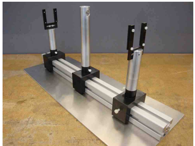
FIG. 15.7 – Telescope to test LGAD.
