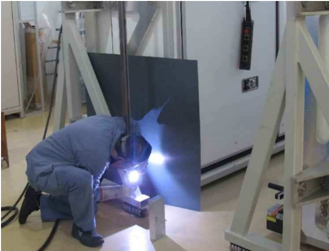
FIG. 15.8 – Welding work for reinforcement of the transportation frame done directly on a FlashCam camera body.
