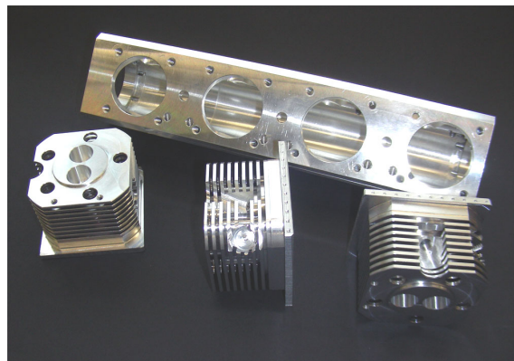
Figure 15.5: Cylinder heads and the crankcase for the V8 combustion engine.
