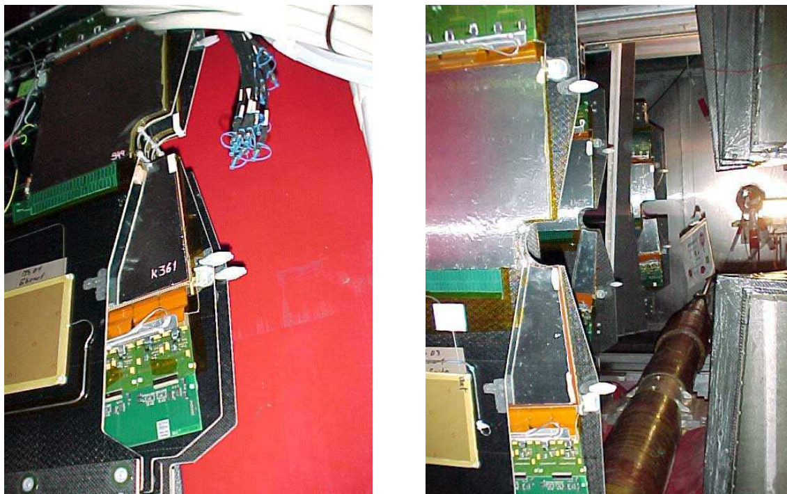
Figure 8.1: Left: view of one half of the first station in front of the magnet. The special arrangement of the different layers allows for an overlap of the detectors. Right: view along the beam pipe in +z direction in the magnet. One can recognize the three stations which are instrumented with MSGC's because of the small cutout for the beam pipe.
