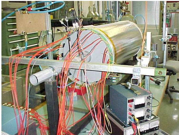
Figure 7.2: The one-third full length prototype of the new CIP being tested in the laboratory.
