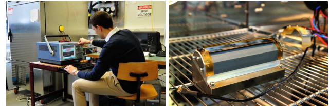
Left: mu3e test stand in our lab; right: detail showing one of the first "ladders" of the mu3e vertex detector.
