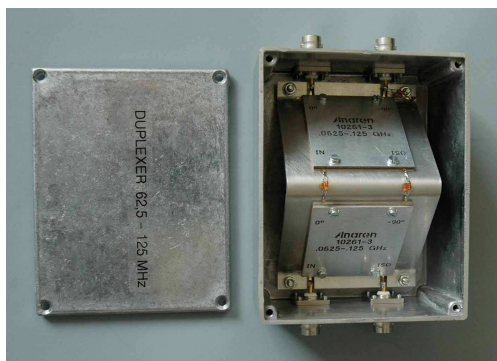
Figure 14.3: Duplexer built for the SCOPES NMR-spectrometers.
