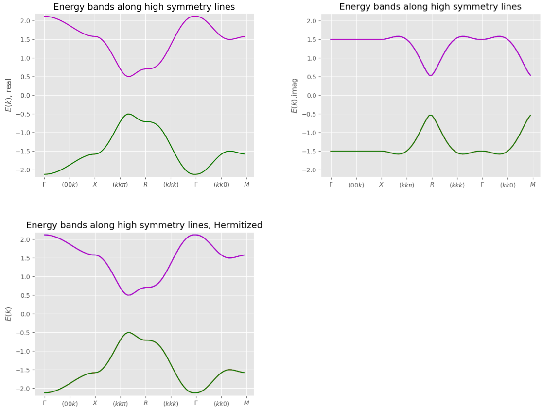
Figure 7.5: Energy bands for nH Hamiltonian along high symmetry lines. Above two plots are the real and imaginary part of the energy. The bottom plot is the energy band for the hermitized Hamiltonian of the above one. As we see the real part of the energy band for nH Hamiltonian is exactly the same as the band for the hermitized model, (H + H^\dagger)/2 and H is the nH Hamiltonian. Lower band of the real energy band corresponds to the lower energy band of imaginary energy and upper real corresponds to the upper imaginary bands.
